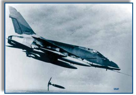
F-100 dropping a Mark 82 "Snakeye" bomb. Note how the deployed fins cause enough drag to slow the bomb, thereby allowing the low-flying attacking aircraft to avoid damage from the resulting bomb blast.
